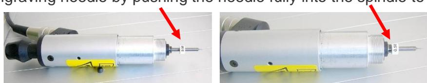
Screw the depth controller onto the spindle.
