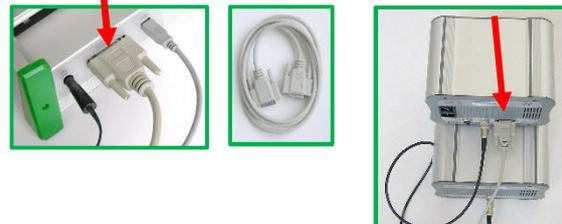
Connect the spindle cable to the Engraver-Controller (EC) and fix it.
