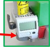
If pressed again for approx. 3 seconds, the counter will change from mm to inch counting and vice versa. If not used for 15 minutes the counter will turn off. Inside the counter you can find a small battery, type CR 2032.
