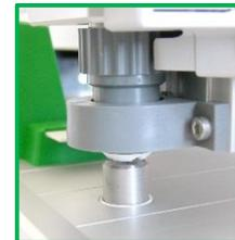
**Note:** If there was no contact made because of the needle not sticking out, the **plotter out of order LED** flashes together with the **STOP LED**. Turn off the power of the plotter, change the needle setting and start again.
