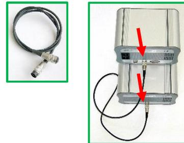
Connect the Engraver-Controller cable between the EMS-3 plotter and the Engraver-Controller (EC), tighten the plugs on each end.
