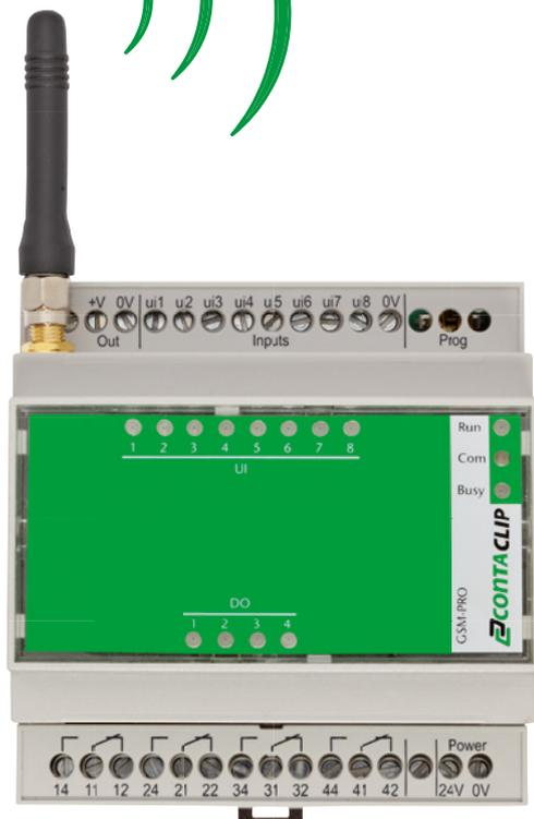
The **GSM-PRO** module features eight multi-function inputs. The input module may be selected as either digital (24 V DC) or analogue (0 to 10V), so that many different signal levels can be connected.
