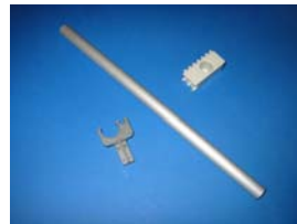
16. Tool for adjusting engraving needle
