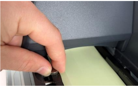
Tighten the locking screw securing the width guides in the right position.
