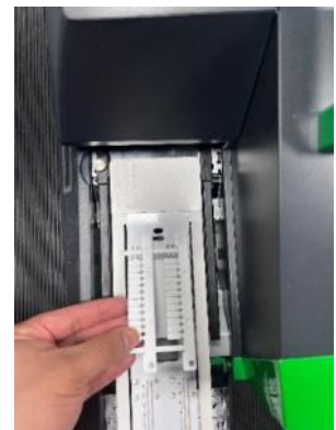
Set half of the card onto the Inlay;
