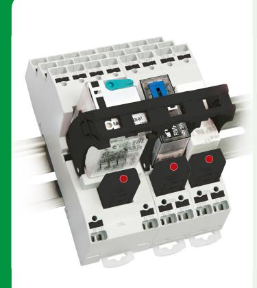
**PPRS** relay sockets with push-in connection are available with two or four CO contacts. The relay sockets are designed for a rated voltage of 300 V. They can be combined with relays and the appropriate insert modules or status displays. In order to guarantee that the relay is mechanically snug in the frame, a relay holding clamp can be mounted.
