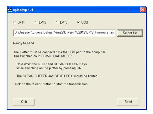
Now switch on the plotter in the download mode. This can be done by holding down the STOP and CLEAR BUFFER keys while switching on the plotter by pressing the ON button. Now the CLEAR BUFFER and STOP LED's should be lit. Click on the `SEND` button to start the firmware update.
